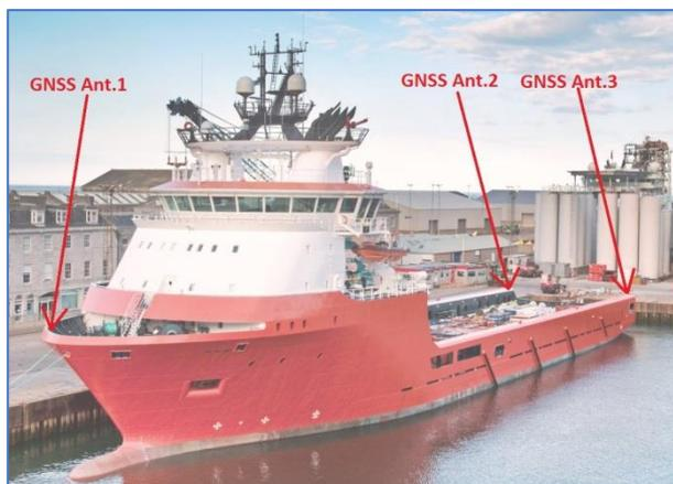
The 3D offsets of the three locations relative to the vessel reference frame are measured only one time through a Total Station in order to ascertain their relative coordinates with millimetric precision.
